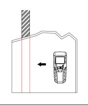
Without releasing on/off button, slide scanner in reverse direction to locate the other edge of stud. Mark this second spot. Middle of stud is centered between the two marks.
