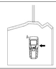
Continue scanning beyond the marked spot to detect width of target. If target is wide, reverse to locate and mark the other edge. Avoid sawing or drilling between the two marks. Widths will vary from single peak for narrow rebar to wide area for metal studs, I beams, junction boxes.
