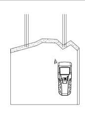
While holding in on/off button, slowly move unit randomly to locate target LCD screen indicates proximity to metal, with center bar indicating closest proximity. Mark this spot.
