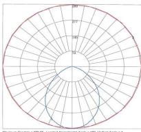
Maximum Candela = 289.05 Located At Horizontal Angle = 180, Vertical Angle = 1 # 1 - Vertical Plane Through Horizontal Angle(s (180 - 0) (Through Max. Cd.) # 2 - Horizontal Cone Through Vertical Angle (1) (Through Max. Cd.)
